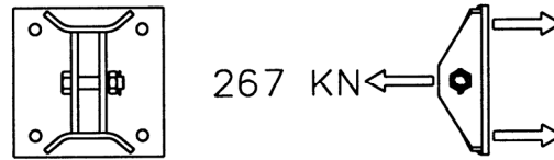
Figure 13—Tensile load test guy plate No. 5
